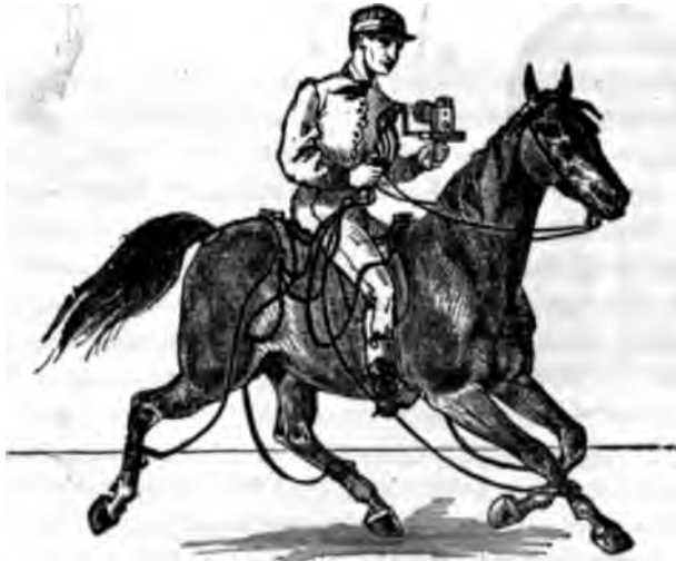
FIG. 177 - Registering apparatus of Marey applied upon the horse at the trot.
